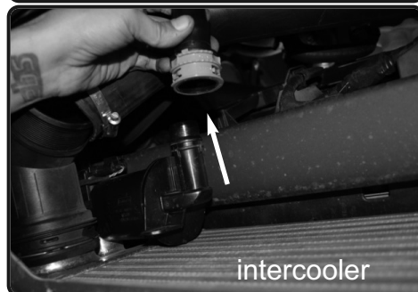
10. Pull back the diverter valve hard line. Twist and turn, pull back.
