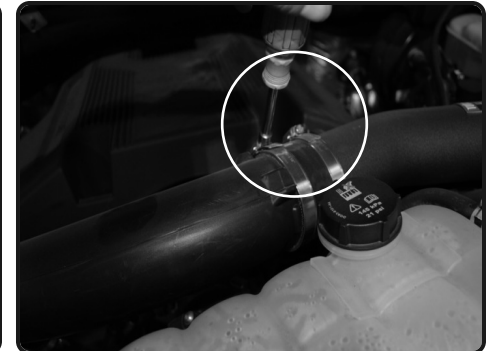
4. Loosen the clamp on the intake system and pull back.
