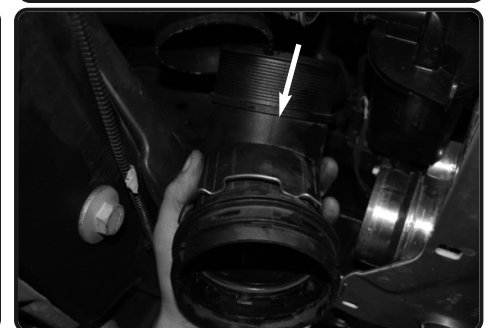
12. Pull back the plastic elbow from the intercooler.
